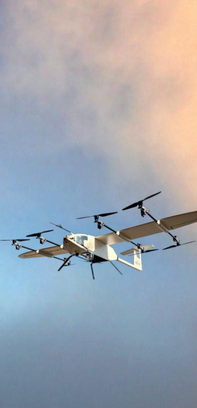
Shifting parts of urban traffic into the air is no longer a dream of the future. Within the Fraunhofer ALBACOPTER® Flagship Project, a flying experimental platform with the vertical take-off and landing capability of a multicopter and the aerodynamic advantages of a glider is to be developed and approved for test and demonstration flights.
